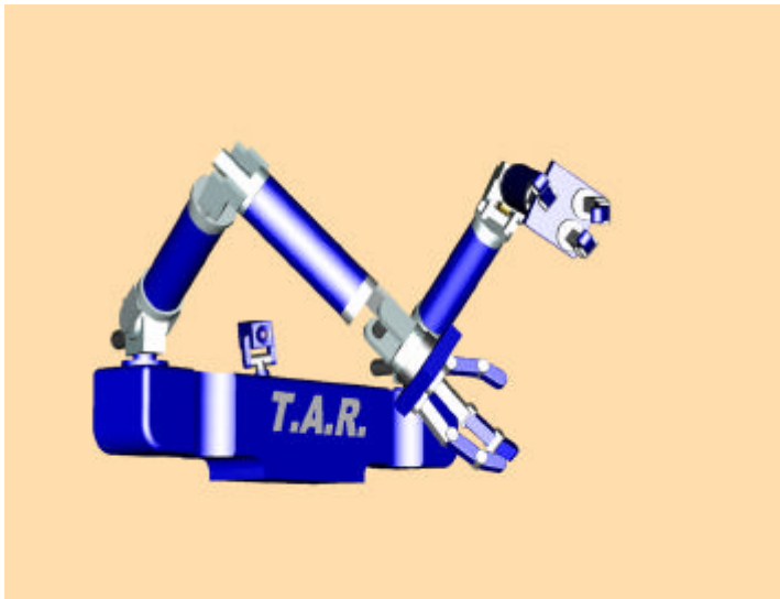
Fig. 1 TAR: Concept for a Two Armed Robot for routine assembly and maintenance tasks on the International Space Station
