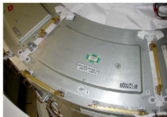
Figure 10: The end-cone Meteoroids and Debris Protection System
