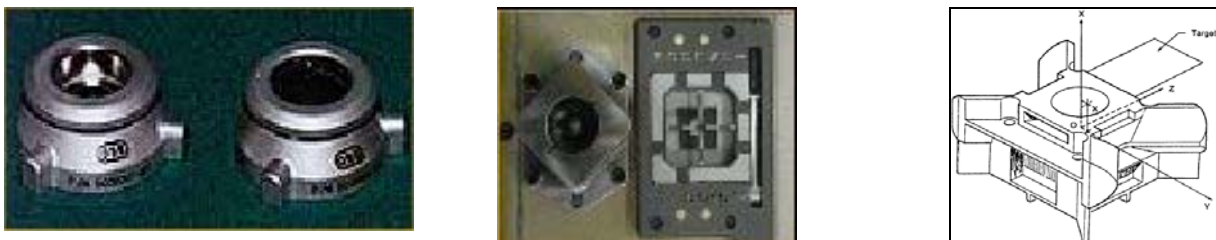
Figure 6: left - Micro-conical fixture; centre – micro-square and its alignment target; right – H-fixture
