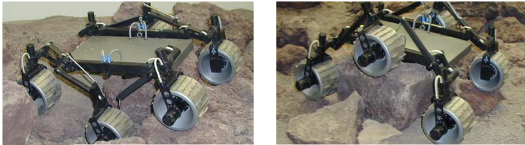
Fig.7 ExoMaDeR model (Concept D) while negotiating rocks (ESTEC A&R Lab)
