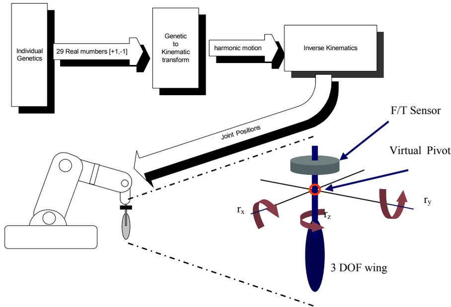
*Figure 3 shows the data conversion necessary to map the genome of each individual to actual wing movement. The genetic to kinematics mapping is processed in the Windows PC, outputting a stream of angular set-points for each of the 6 servos in the robot as to produce the corresponding wing movement. These set-points are then transmitted by serial line to the DOS PC that double checks it for safety and starts the actual motion.*
