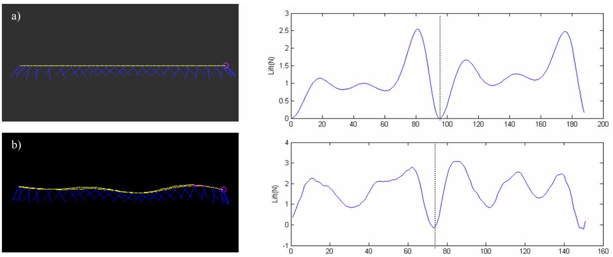
**Figure 4** shows one of the evolved patterns featuring some oscillatory behaviour *b*) compared with the same movement in which the oscillatory behaviour were manually deleted *a*). The oscillations create force peaks in the middle of the stroke, boosting the lift in about 15%, and enhancing repeatability.
