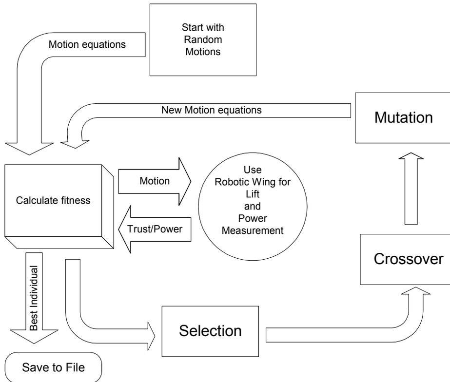
**Figure 2** shown the data flow related to the Genetic Algorithm optimization. Each individual in the population has 29 motion describing genes (29 real numbers) that are converted to wing motion, tested for power/lift, graded according to performance and fed-back to the GA computation. This ranking will affect the processes of natural selection, crossover and mutation. After which the new population is tested again, completing the cycle.
