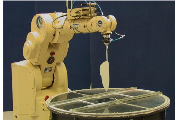
**Figure 1:** View from the robotic setup with wing outside the water tank
