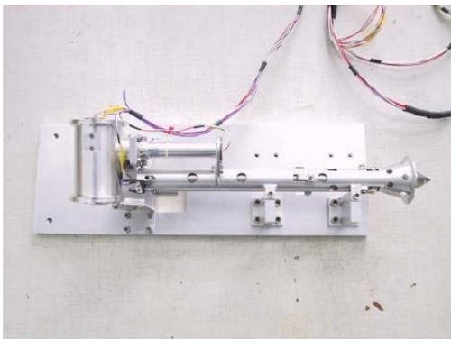
Fig. 5: PLUTO Mole system Qualification Model (with winch mechanism and launch tube); overall length from Mole tip (right) to reel housing is 365 mm.
