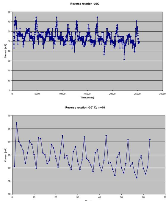
Fig. 6: Recorded PLUTO Flight Model Mole motor current at  $-30^\circ\text{C}$  during reverse rotation (i.e., lead screw extension) acquired at 50 Hz (top) and filtered data (bottom) as required for real-time control.
