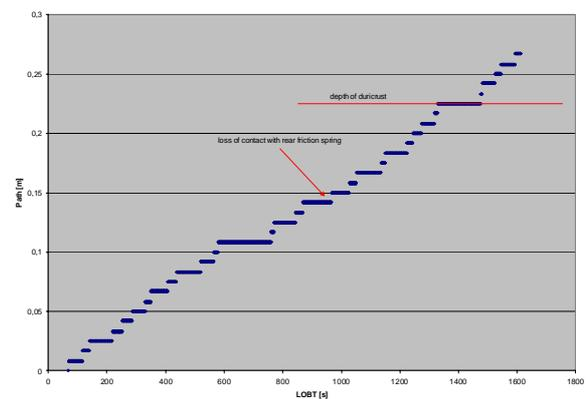
Fig. 7: PLUTO winch count data as function of time as acquired by 'Beagle 2' Ground Test Model electronics and S/W during Mole penetration experiment with layer of simulated duricrust.
