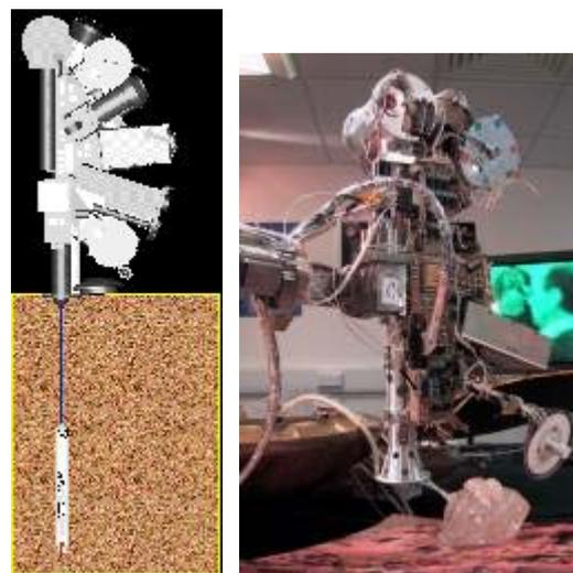
Fig. 1: Schematic (left) and actual mounting of Sampling Mole System on instrument carrier on ‘Beagle 2’ mechanical arm. Left hand view also shows Mole deployment with unreeled tether.
