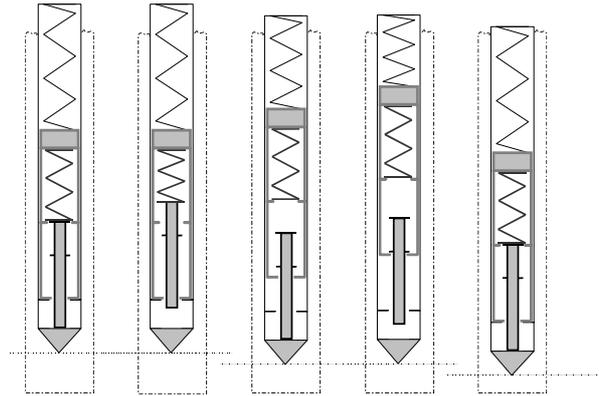
Fig. 2: Principle of Mole forward hammering.
