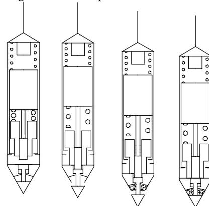
Fig. 3: Schematics of sampling head opening.
