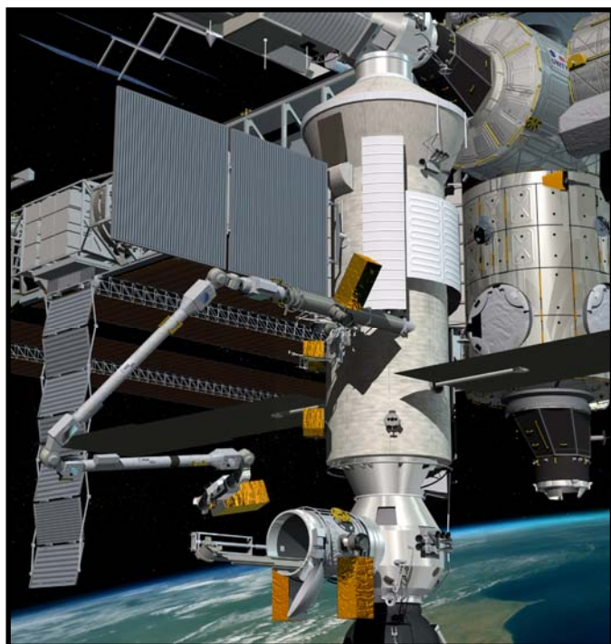
Fig.5, ERA moving a payload from the equipment airlock located on the MLM
