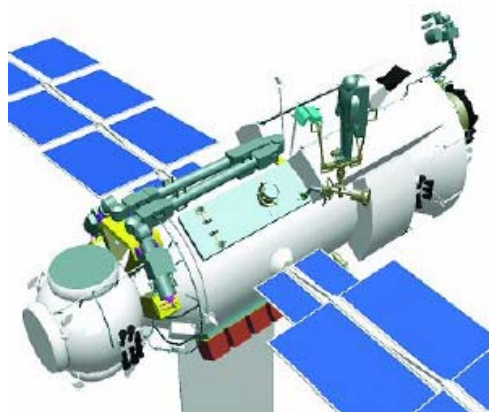
Fig.7, ERA on the MLM at the start of the In-Orbit Validation
