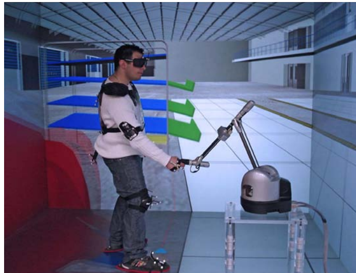
Fig. 2: Ergonomic study for vehicle assembly (courtesy PSA Peugeot Citroën)
