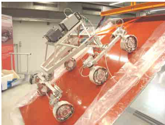
Figure 3. Static stability test on a 40° slope
