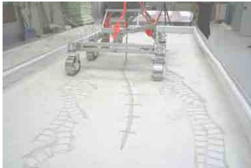
Figure 14. path following on leveled surface
