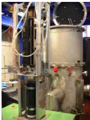
Fig. 17: Drill box integrated on the supporting structure before installation within the T/V chamber
