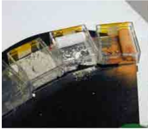
Fig. 19: Samples discharged into the container (from right: red brick, marble, regolith)
