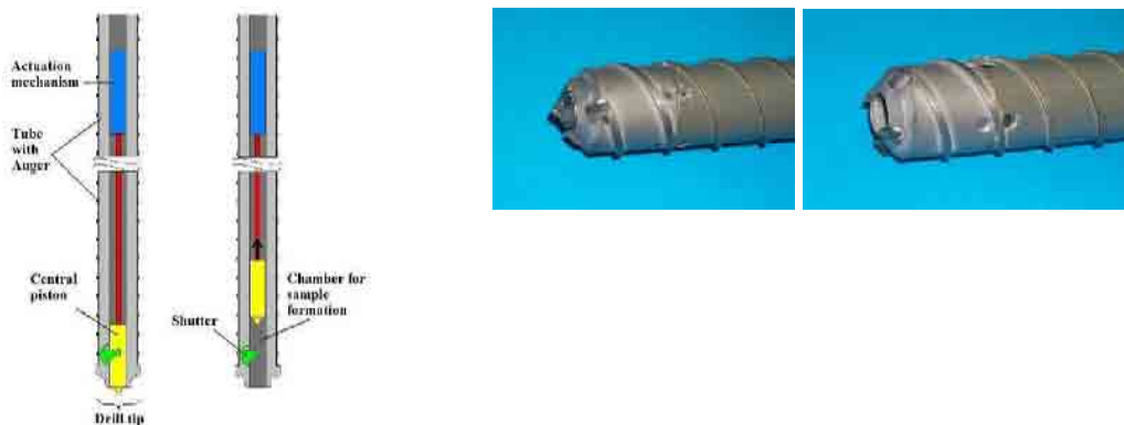
Fig. 6: Drill tool schematics on the left and drill tool BB
