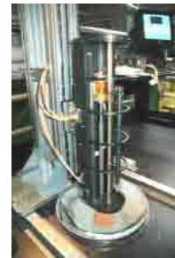
Fig. 14: Drill box with drill tool and ext rods integrated for the 2 m depth test
