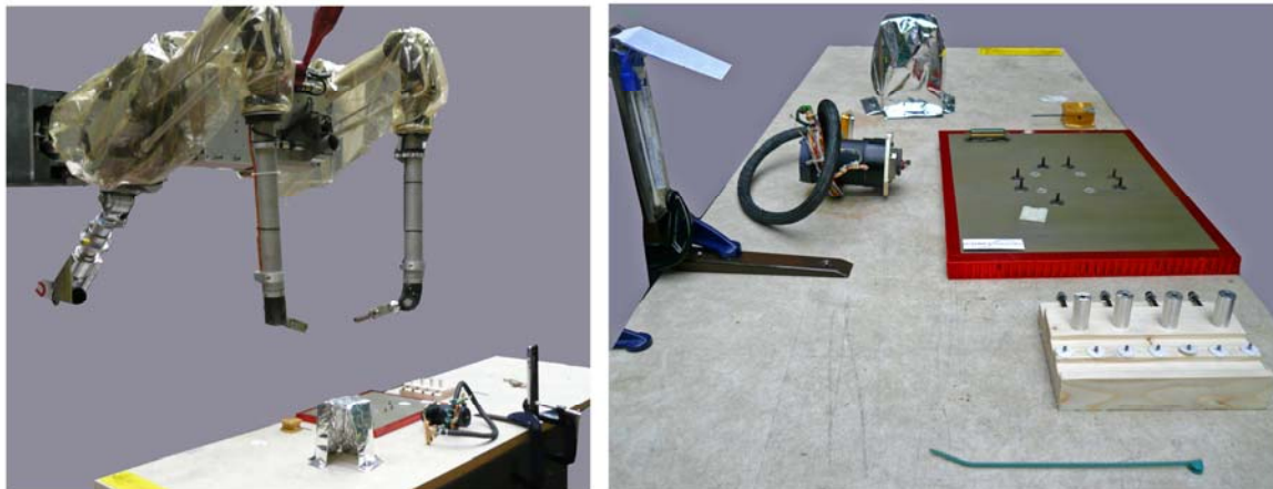
Figure 1 – Dexter Manipulator with AIV Mock-up (dis-assembled)
