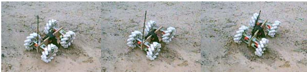
Fig. 17. Driving through a “crater”. The rover traversed the crater in 12 seconds.
