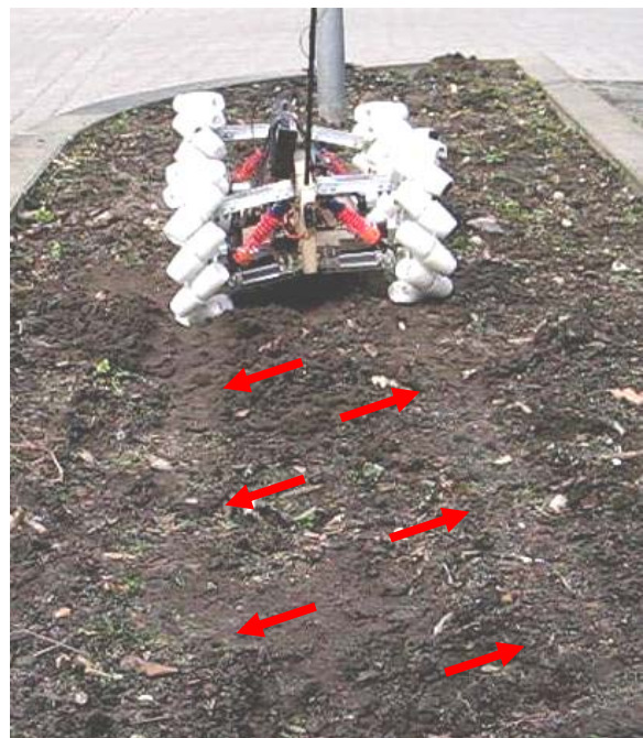
Fig. 14. Rover driving over very rough terrain. Arrows mark the vehicle's tracks
