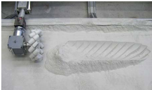
Fig. 7: Mecanum wheel subjected to a load of 15 N (90° wheel orientation).
