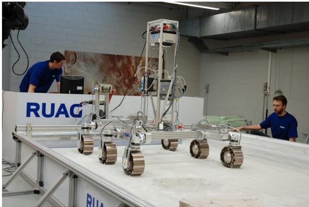
Figure 2. ExoMars LSS Breadboard 2 in the RCET Testbed (RUAG Space, Zurich)
