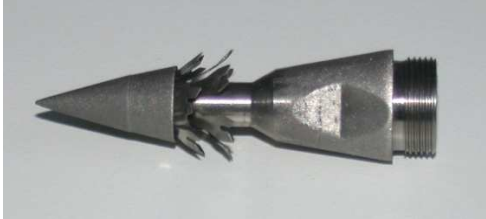
Figure 5. Titanium tip with two rows of barbs
