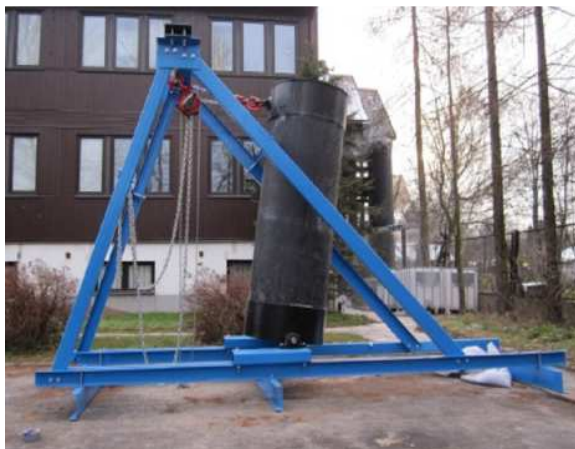
Figure 10. The 1.8-meter test-bed system with variable inclination.
