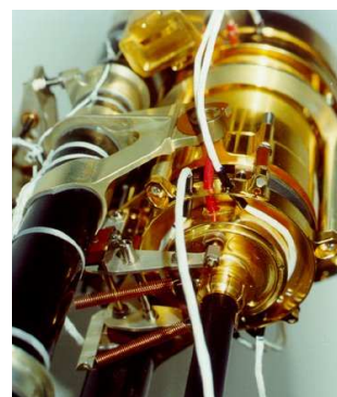
Figure 4. MUPUS hammering Insertion Device integrated on the EQM model
