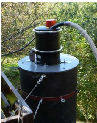
Figure 8. The top of the 5-meter test-bed with vacuum conveyor
