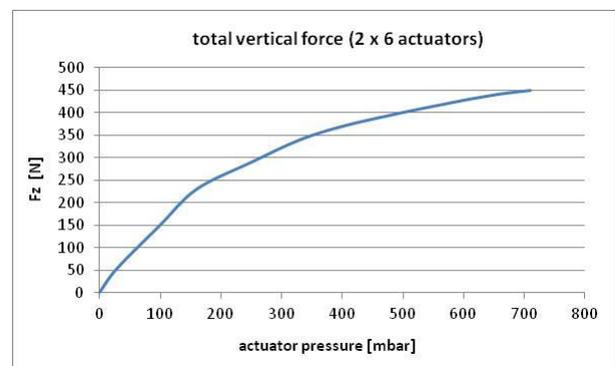
**Figure 8: Vertical force  $F_z$  between the shoulder and the crotch as a function of the sigma actuator pressure.**
