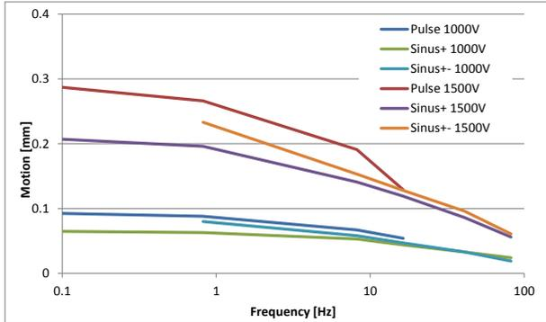
**Figure 4: Peak deformation (motion) in dependence of the actuation frequency**
