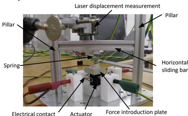
**Figure 3: EAP stack actuator demonstrator setup.**
