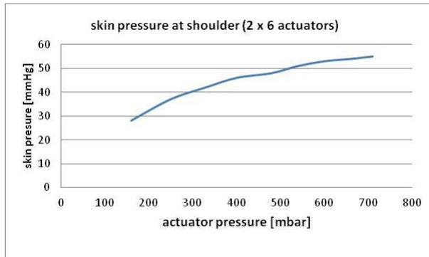
**Figure 9: Skin pressure at the shoulder as a function of the sigma actuator pressure.**
