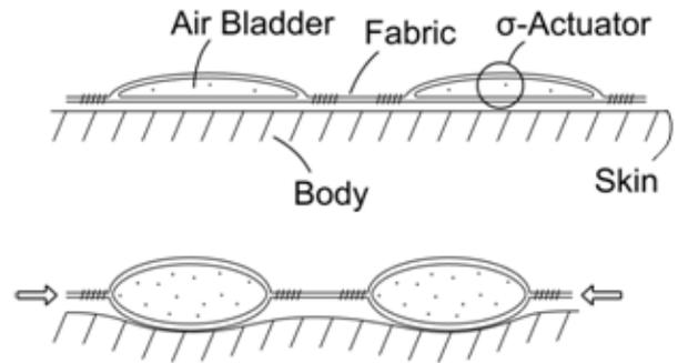
**Figure 6: Cross sectional view of two sigma actuators in the relaxed (upper) and activated stated (lower).**
