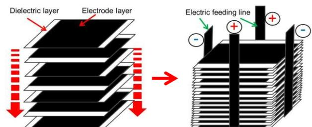
**Figure 2: Assembly of the multilayer system and attachment of the feeding lines.**
