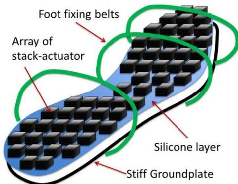
**Figure 1: Arrangement and interface design of the EAP actuators for foot sole stimulation.**
