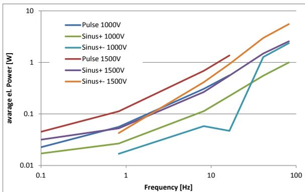
**Figure 5: Power consumption of one stack actuator as a function of the actuation frequency.**
