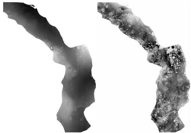
Figure 4. Left: DEM of whole test site (length approximately 400m) generated during the trials from aerobot images. Right: Corresponding ortho image.
