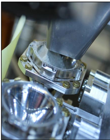
Figure 13. Close-up of PSDDS sample inlet hopper with crushed ‘coarse sand’ having accumulated (outlet funnel of CS is visible at top)
