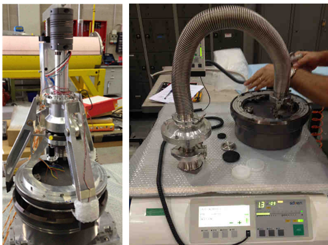
Fig. 16 Lid closure test (left), leak rate test (right)
