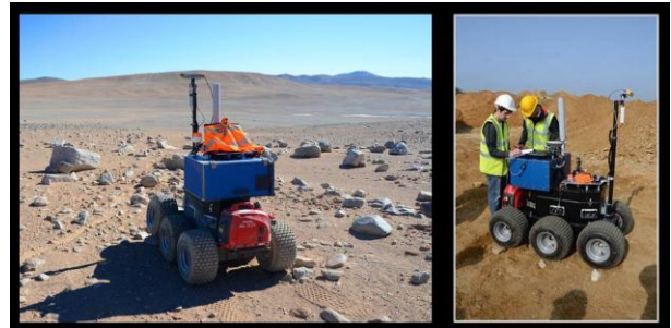
Figure 10: SEEKER platform –Robovolc provided by BAE Systems. Bumblebee Stereo-pair mounted on the forward facing mast. Generator for extended operations mounted on the rear of the vehicle. DPGS (ground truth testing) and Wi-Fi antenna in the centre
