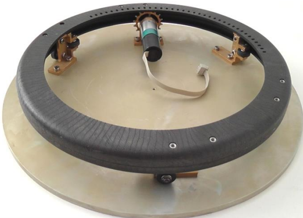
Figure 11. Rotational joint mechanism fixed on the baseplate. The ring can withstand 300N loads.
