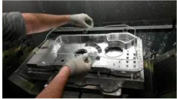
Figure 18. Fit check of UCZ pressure seal (Inconel C-ring type) on baseplate of STM of ALD structure, April 2015
