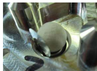
Figure 5. Dispensing test with blank sample; metal foil at blister package bottom has torn along engraving pattern
