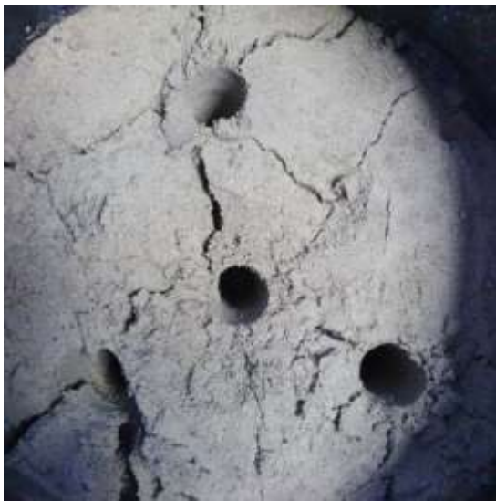
Figure 20. Icy regolith sample following strength testing by penetrometer
