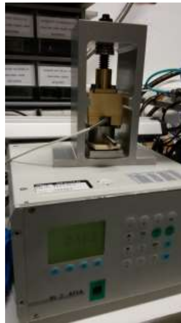
Figure 21. Test set-up at OHB for measuring ProsPA oven sealing forces and leak rates
