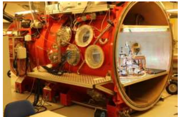
Figure 16. E2E ‘phase 2’ testing in Mars environmental conditions: scene from March 2013 at Aarhus test facility, E2E test set-up is visible on chamber bottomplate
