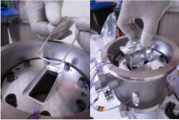
Figure 10. Breadboard testing of ALD door with metal C-ring seal (May 2014)
