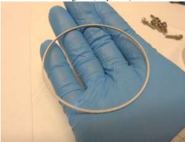
Figure 11 : One of the Inconel C-rings used in the SPDS as a static seal
