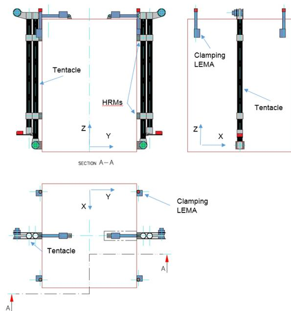
Fig. 3: Sketch of the stowed mechanism concept
