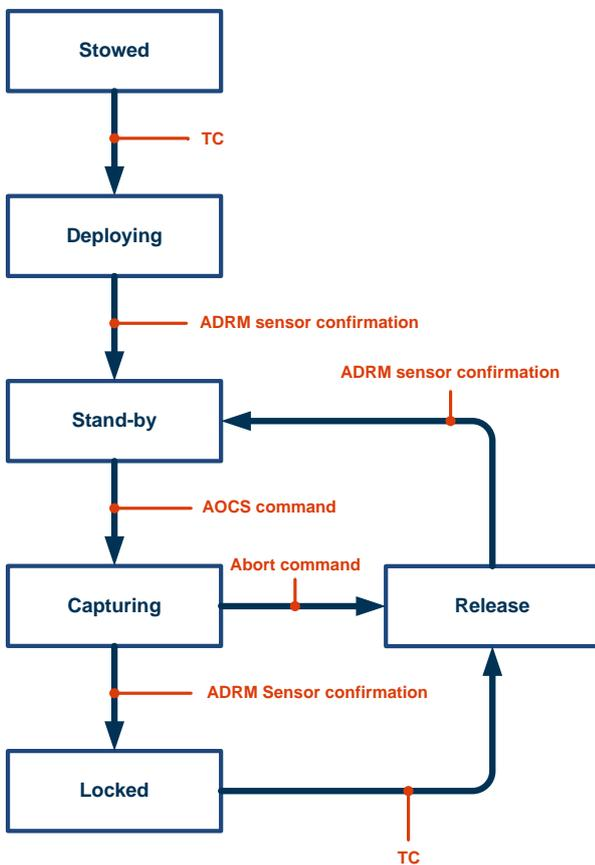
Fig. 1: Clamping mechanism state diagram
