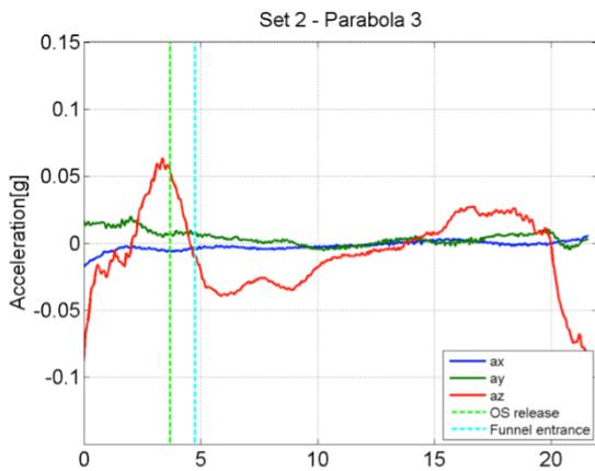
Figure 11: 2nd day, 2nd set, 3rd parabola: Microgravity phase accelerations
