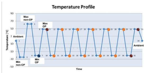
Figure 2: TVT thermal cycles.
