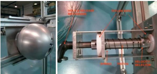
Figure 3: OS launcher.
