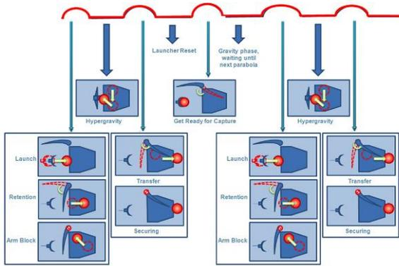
Figure 6: Complete test schematics.
