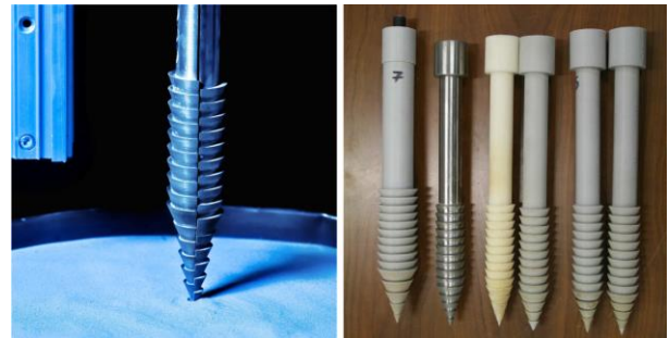
Figure 3. Pictures of the DRD (left) and the various mono-block drill heads (right) used in experiments detailed in [8] and [9] respectively
