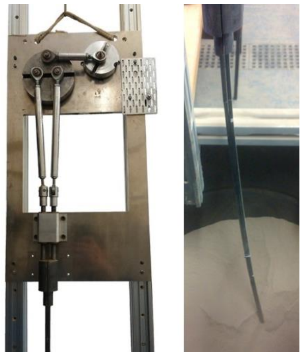
Figure 4. Pictures of the proof of concept test bench (left) and the bent drill stem after taking a curved trajectory whilst drilling (right)
