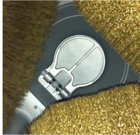
Figure 5. Sample Canister door mechanism
