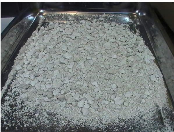
Figure 11. 300g of sampled regolith simulant (sepiolite from 1micron to 3cm)
