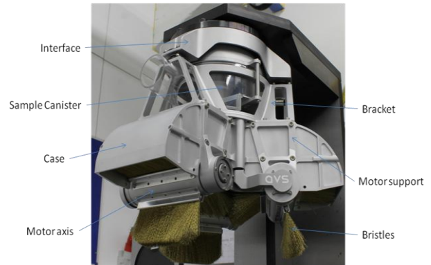
Figure 2. AVS Sampling Tool Mechanism Breadboard
