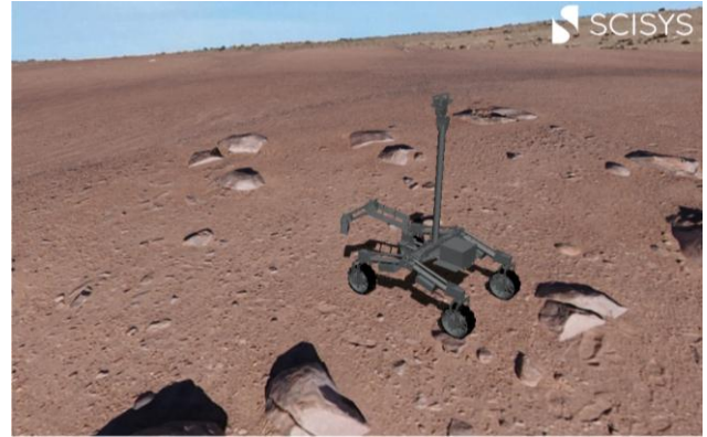
Figure 6: SOLO Rover visualised in Overseer INTERACT using 5mm resolution terrain model reconstructed from UAV data.
