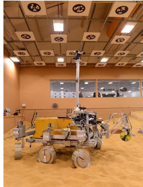
Figure 3- Airbus DS Bridget Rover platform carrying the FASTER Wheel Bevameter sensor on a deployable arm at the front
