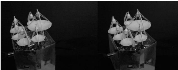
Figure 1 Two images taken from a Satellite mockup (test set-up) at different positions of the camera
