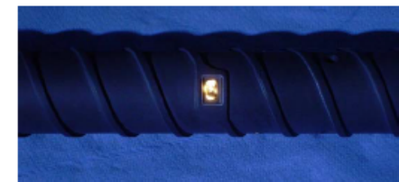
Lamp lit and the light conveyed via optical fibre and optical prism through the sapphire window (taken over a dark background)
