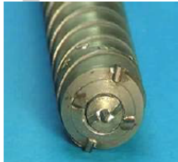
Drill Tool with Central piston in "Drill Mode"
