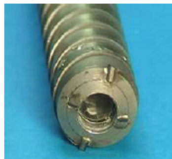
Drill Tool with Central piston in "Core Mode"
