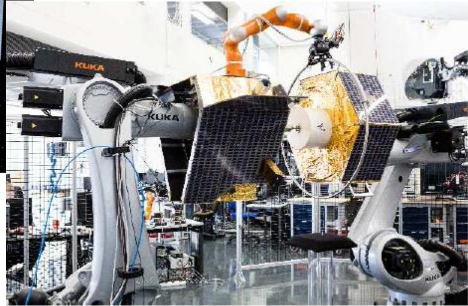
On-ground scenario two industrial robots and a Light Weight Robot (LWR) – chaser (left) and target (right) – DLR OOS
