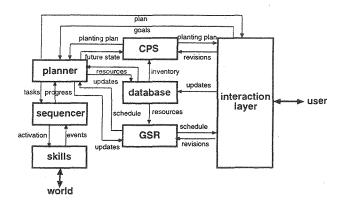
Figure 1: The complete planning, scheduling and control architecture for advanced life support systems.
