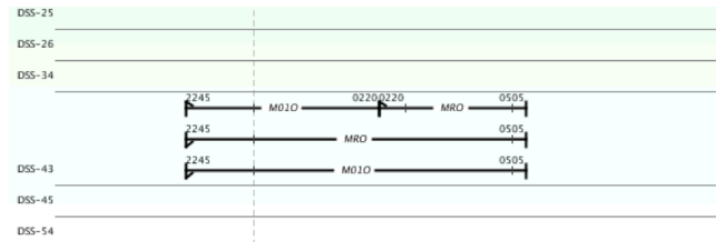
(a) An example S 3 MSPA grouping on DSS-43 where the uplink-only and downlink-only tracks are represented separately. Two spacecraft (MRO and M010) are downlinking simultaneously while the uplink occurs for M010 at the beginning of the track, then transitions to MRO until the end of the track. The equipment specified for each track represent just those that are needed to support the uplink and downlink services individually.
