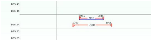
(c) An example of an Multiple Track Reconfiguration conflict. If the two tracks are merged together into a legacy track, it would begin as downlink-only, reconfigure to uplink and downlink at 0415, and then reconfigure again at 0845 to downlink-only. There is a limit of only one track reconfiguration for MSPA tracks
