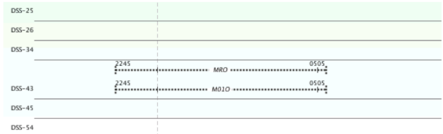
(b) The same MSPA grouping example as in Figure 1, but represented in the “legacy” track view. In this view, the uplink and downlink tracks are merged together and the activity description field contains the track reconfiguration times and supporting equipment needed.
