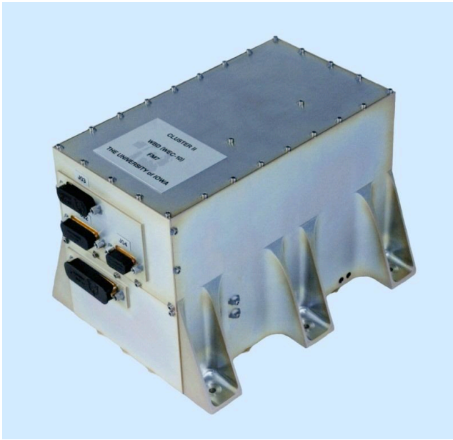
Figure 5. The Cluster II Wide-Band (WBD) plasma wave receiver. One such instrument is on each of the four Cluster spacecraft.
