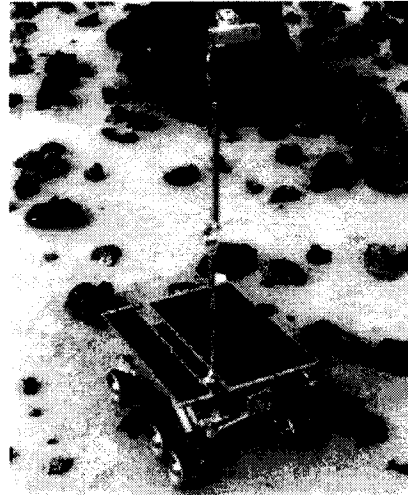
Figure 1: The Rocky7 Prototype Microrover, developed at JPL to test technologies for future missions. It is pictured here in the JPL MarsYard, an outdoor testing arena featuring simulated martian terrain.
