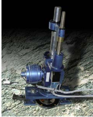
Fig.2: Prototype Planetary Drill Electric Vehicle Controllers Ltd.
