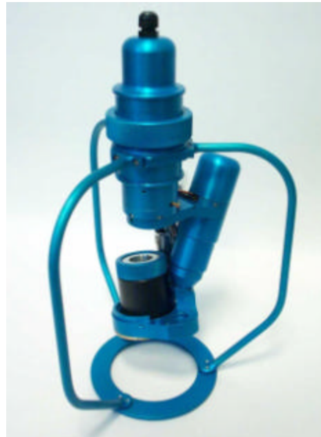
Figure 3 : The 4 degree-of-freedom light robotic probe holder developed under contract funded by ESA 2000
