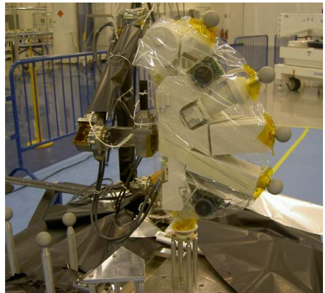
Figure 14: FM ARM and 1/3rd mass PAW shown after being commanded to position the mole in the GAP inlet port using Envision(TR) generated ARM joint data.
