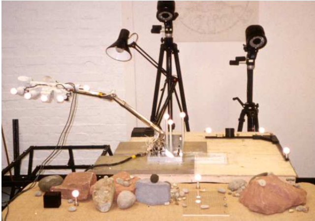
Figure 3: Calibration setup with the Beagle2 Development Model (DM) ARM, 1/3rd mass PAW, and mock terrain.
