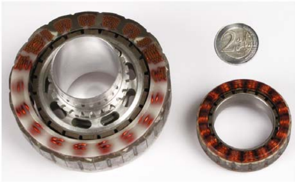
Fig. 7 Two sizes of ROBODRIVE (ILM 85 with 1.4 Nm torque and ILM 50 with 0.3 Nm torque)
