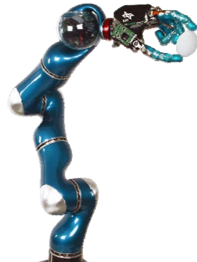
Fig. 25 DLR's operational light-weight arm/hand system
