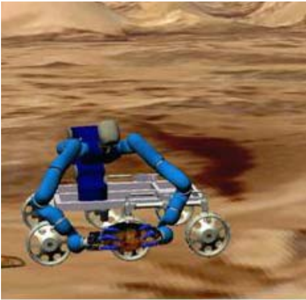
Fig. 27 A humanoid planetary rover concept based on DLR's light-weight arm/hand system
