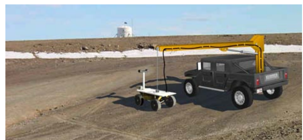
Fig. 10, Artist's rendition of lunar energetics experiments conducted using a gravity compensation system.
