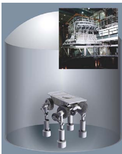
Fig. 9, Artist's rendition of the lunar rover chassis in a test fixture in a thermal vacuum chamber to emulate the lunar environment for testing.
