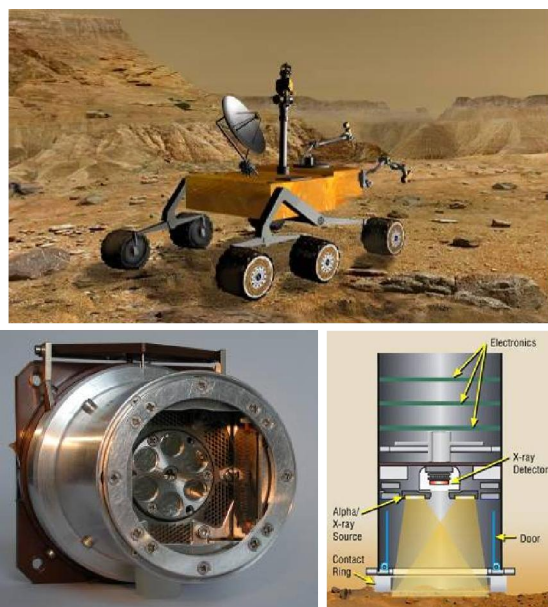
Fig. 10. NASA's Mars Science Laboratory (MSL) and MDA's Alpha Particle X-Ray Spectrometer (APXS)
