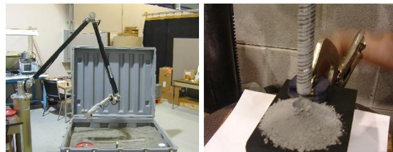
Fig. 13. Exploration Arm Scoop and Drill Bit testing in regolith simulant
