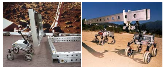
Fig. 7. Left: RCC carries a panel and aligns with the structure. Right: RCC carries a beam outdoors.
