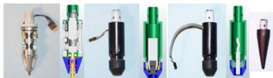
Fig. 11. LEMUR tool set, left to right: rotary driver, camera, flash light, foot/pointer.
