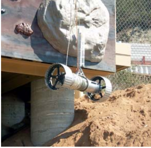
Figure 9. Axel lowered over a simulated promontory mounted on the viewing platform in the JPL Mars Yard.
