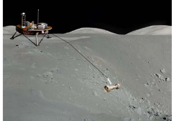
Figure 1. Conceptual rendition of the Axel tethered rover on the Apollo 17 landing site background (picture not to scale)
