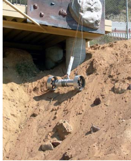
Figure 10. Axel driving down a 40° rocky slope in the JPL Mars Yard
