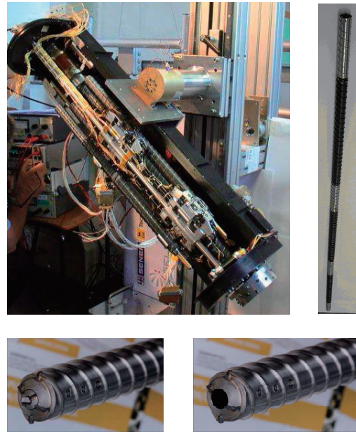
Figure 5 Developed Drill and Sampling System H/W
