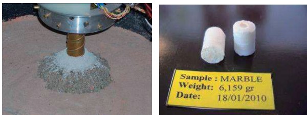
Figure 17 Typical heap formation and a sample collected during integrated testing
