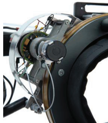
Fig. 5: Overview of the direct-drive unit in axis 6 (for upper arm rotation). The torque sensor measures the reaction-torque on the motor casing instead of the direct output torque (since the arm passes through the middle of the joint). To remove influence of motor mass on sensor readings, an additional mechanical decoupling structure is included. Thus, the sensitivity of the torque sensor was significantly increased.
