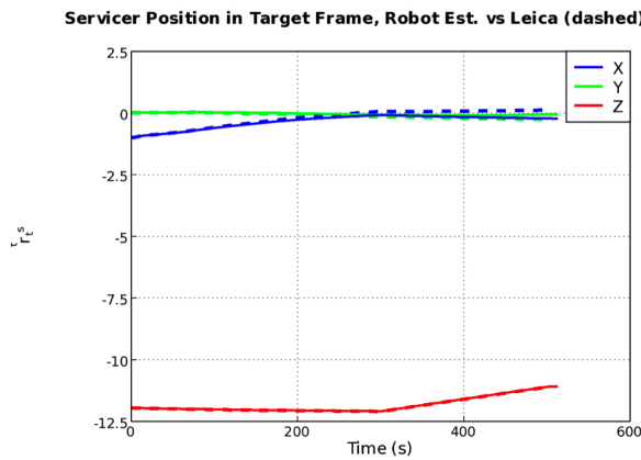
Figure 15. Argon position in target frame, test 93, spinning target; Leica relative measurement.
