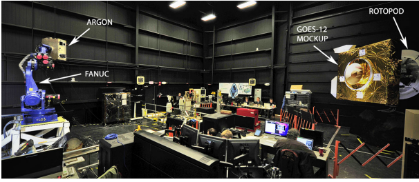
Figure 1. NASA/SSCO relative navigation satellite ground simulator.
