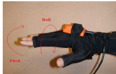
Figure 5 – Arrangement of third accelerometer
