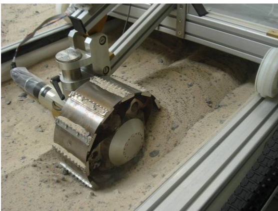
Figure 12. ExoMars BB2 wheel test at 300N load, 70% slip on ES-3
