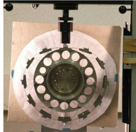
Figure 4. Flexible wheel characterisation bench measuring the stiffness of the ExoMars BB2 wheel
