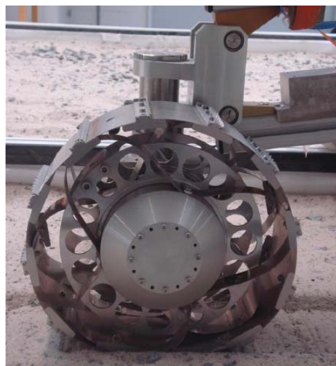
Figure 10. ExoMars BB2 wheel side view, 300N load, 5% slip on ES-3
