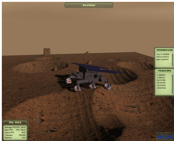
Figure 2: The OGRE based 3-D visualization showing a motion sequence of the ExoMars rover which was simulated with RPAT.
