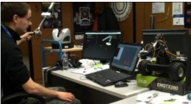
Figure 2 - Rover Robotic Arm (small-scale model) controlled by Haptic Device
