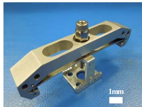
Fig.5 Hopping examination model of the buckling bimetal actuator (with additive 5.0g mass)
