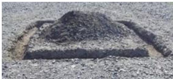
Figure 2. Artificial structure (a castle) for testing MRPTA mapping capabilities
