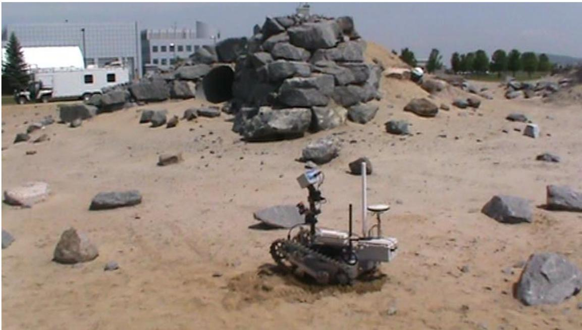
**Figure 8 – MRPTA moving across the CSA Mars Yard along the delivery demonstrations**
